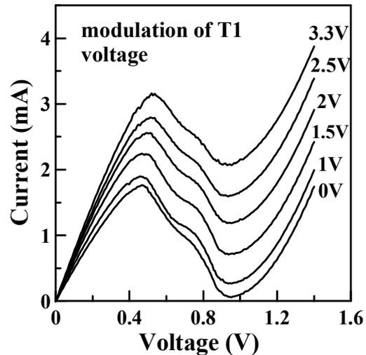
Fig. 8 The peak current of the NDR I-V curve can be controlled by the magnitude of T1 voltage
