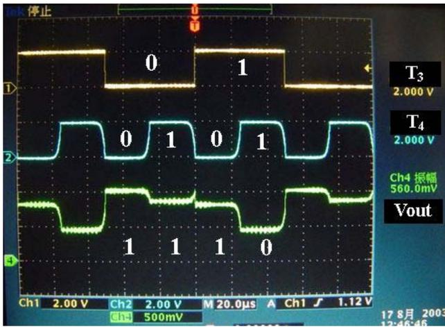
Fig. 10 The measured result for the NAND gate operation.
