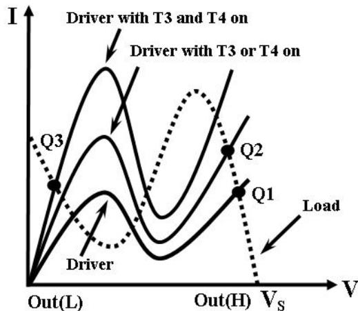
Fig. 7 The load-line analysis for the NAND gate.
