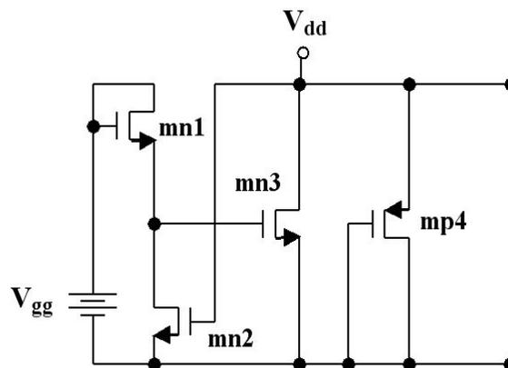
Fig. 1 The circuit configuration for a MOS-NDR device.
