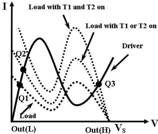
Fig. 6 The load-line analysis for the AND gate
