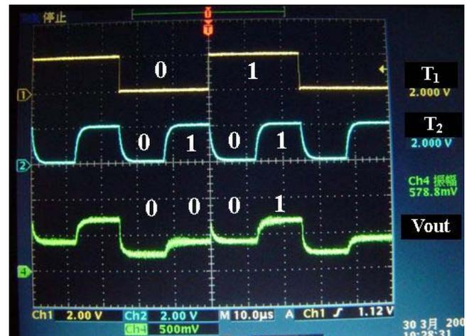
Fig. 9 The measured result for the AND gate operation.
