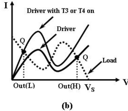
Fig. 5 The load-line analysis for the (a) monostable case ( $V_S < 2V_P$ ), (b) bistable case.
