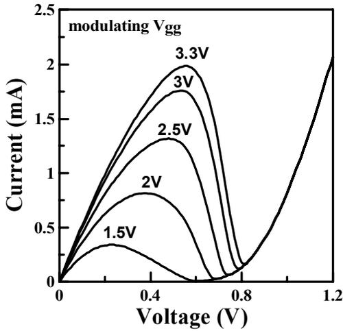
Fig. 2 The Hspice simulated I-V characteristic for a MOS-NDR device by modulating the  $V_{gg}$  values from 1.5V to 3.3V.
