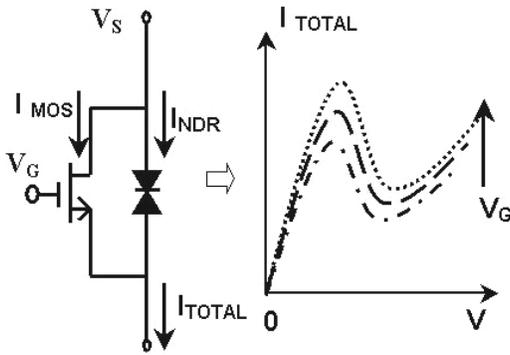
Fig. 3 The peak current of MOS-NDR device could be controlled by the  $V_G$  voltage.
